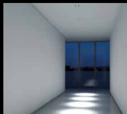
20° Narrow Beam Spotlights, projected onto the floor as "circles of light" illustrate how they can be used to guide movement.
