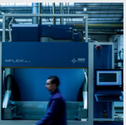
Laser micro-etching machine for PMMA.
