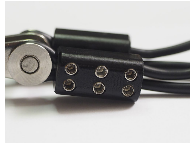
Above: Tighten and secure grubs screws until they are flush with the fixing blocks.
