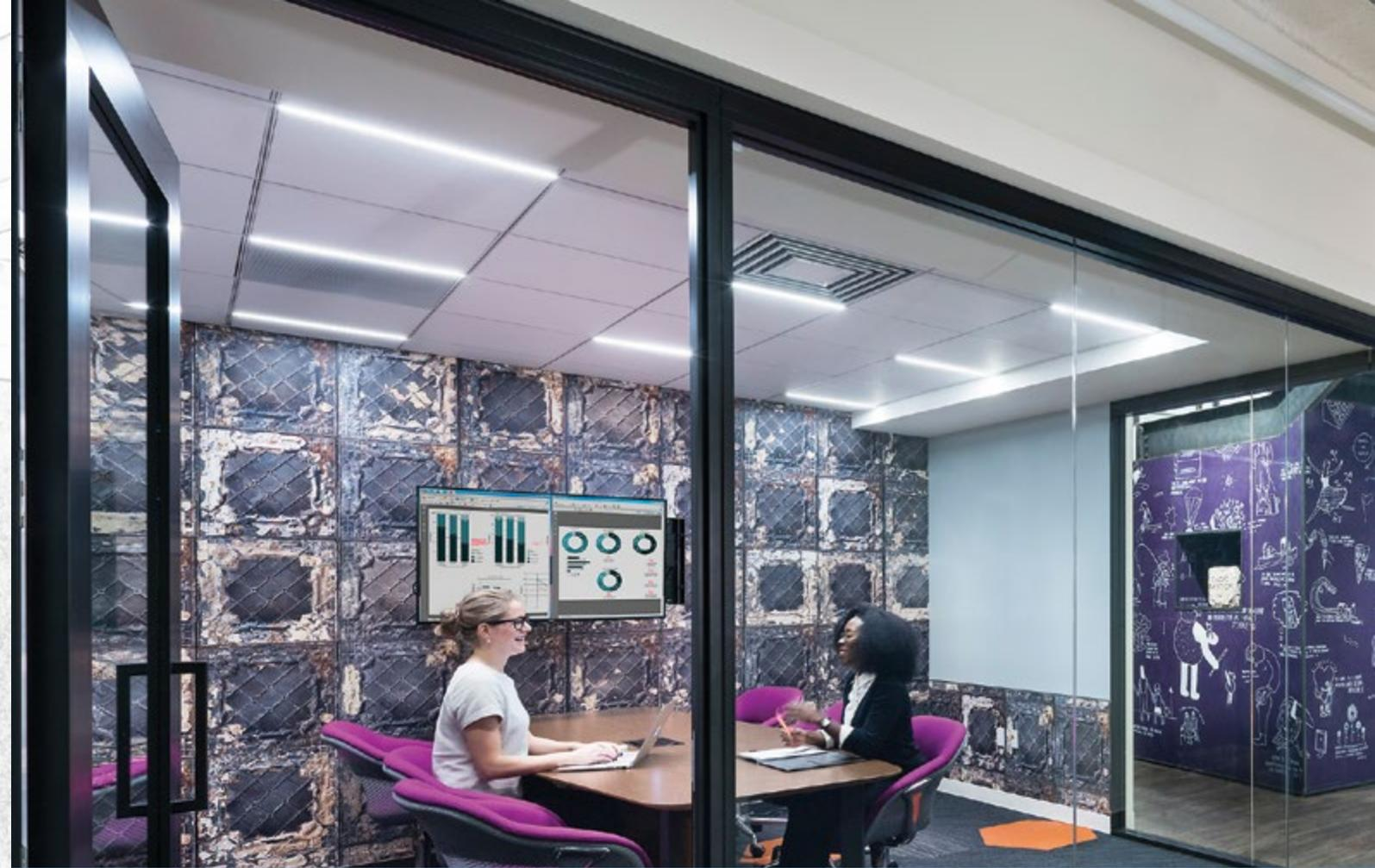
*“There are many reasons why we chose to use the T-BAR LED fixtures, and probably none more than acoustics. This client was very sensitive to sound transfer between enclosed spaces, and the T-BAR LED was a big part of our solution. Having the fixture integrated into the ceiling grid system allows additional ceiling tiles to be installed to absorb sound, and also to limit sound transfer through the light fixture, which is not the case with a traditional 2x2 fixture.”*
