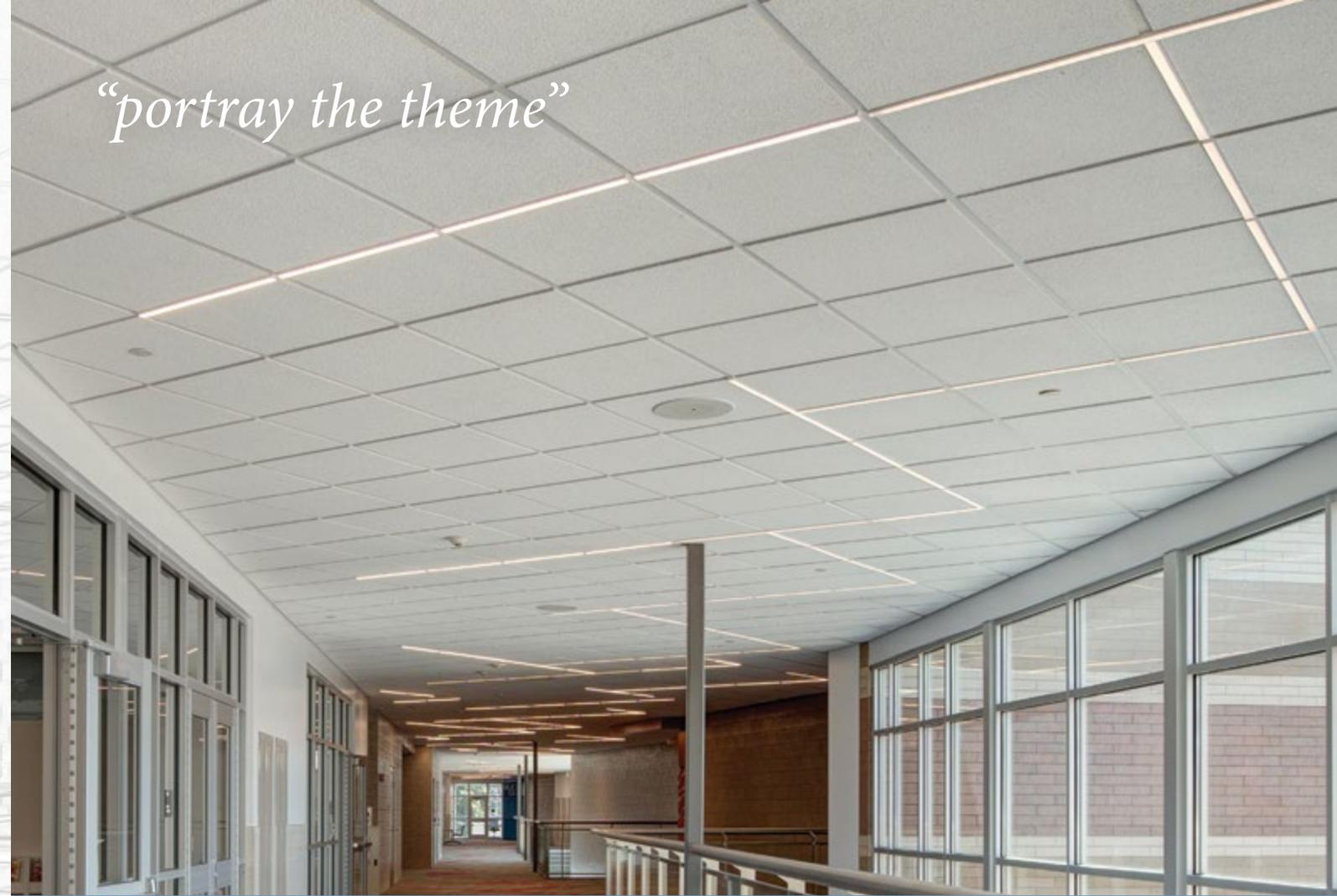
*“The theme of this School was Mountains and Valleys. The Architect wanted to portray the theme into the main corridors of the building. The T-BAR LED lighting system was used to create the mountains and valleys in the corridor ceilings using a rotated ceiling grid layout. The lighting system did a great job illuminating the corridors and stairwells without cluttering the ceiling and creating the ‘Mountain and Valley’ look.”*
