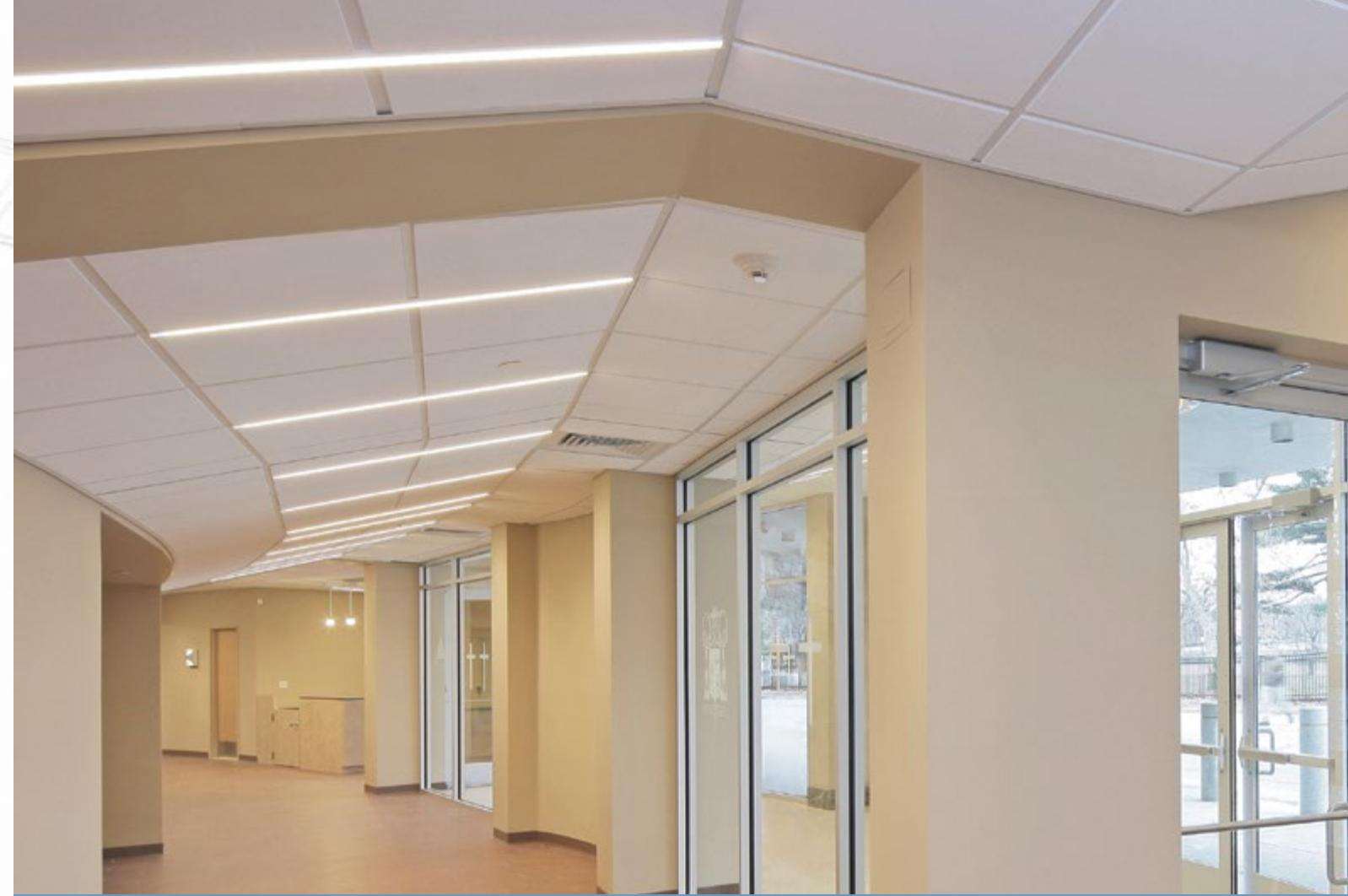
*“The raked ceiling and the T-BAR system allowed us to provide the general area lighting that we needed along with the marquee sparkle that every Theater desires for an entrance. The rake was important for the architectural effect as it made the lighting itself more visible. The T-BAR’s low profile proved to be the one lighting system that could achieve both effects.”*
