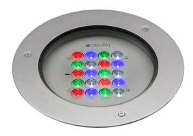
Featuring shallow recessed depth for a comfortable in-ground installation, RUBY R is a highly performing LED fixture specifically designed for exterior recessed applications. This compact IP67 rated light fitting features a 2000 Kg deadweight load capacity that makes it suitable for ground mounting applications even in vehicular areas.
